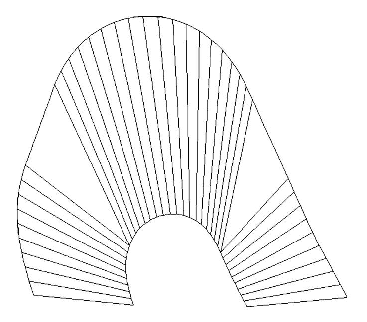
It is possible to cut out the shape and connect the two ends together to flatten the curve.
